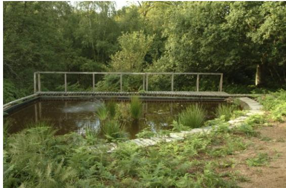
**Lower Pond.** Because of the risks associated with the structure of the upper pond, a second pond was excavated further down the slope, also with a butyl liner, in the form of a shallow bowl, 5 or 6 feet deep in the middle; but with shallow slopes at the edges, not posing significant risk to children were they to fall in. This pond was excavated by machinery after my gap student that winter went on strike over the scale of the task!
